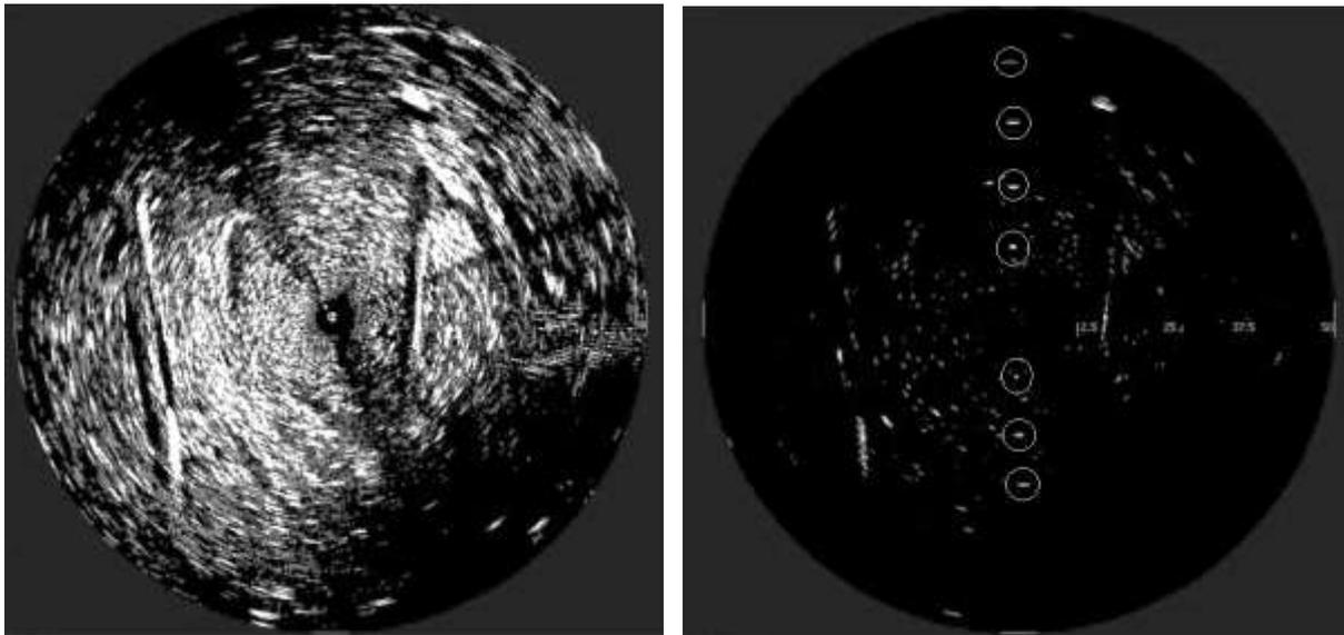
*Figure 12. An example of the sonar picture of the line of SonarBell; (left) image of line of SonarBell and (right) same image with sonar sensitivity reduced, positions of SonarBell highlighted by circles.*
