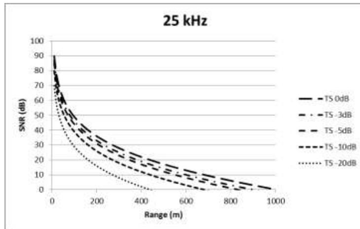
Figure 3. Plot of received SNR against operating distance for reflectors with different target strengths operating at a frequency of 25 kHz and  $NL = 70$  dB re  $1\mu Pa$ .
