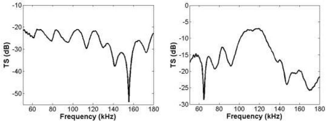
Figure 9. Calibrated amplitude response of a 200 mm SonarBell optimised for 120 kHz; (left) specular echo and (right) secondary echo.
