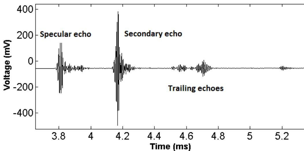
Figure 8. Raw received echo from a 200 mm diameter SonarBell using an LFM pulse.
