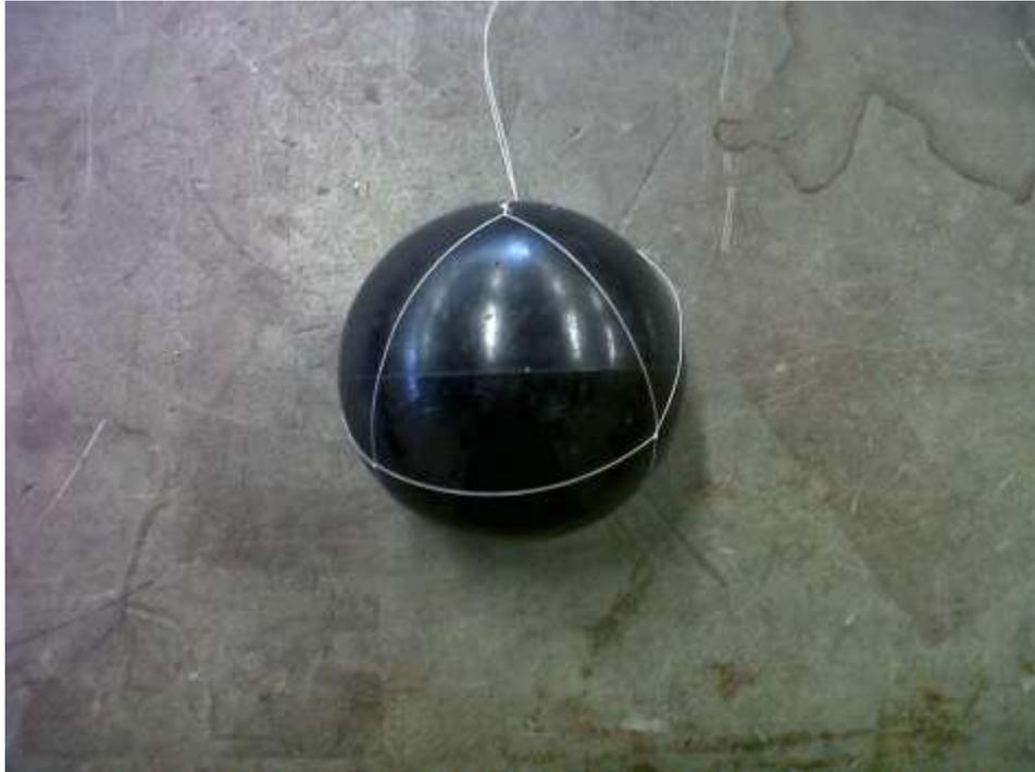
Figure 7. Calibrated 200 mm diameter SonarBell and supporting net.
