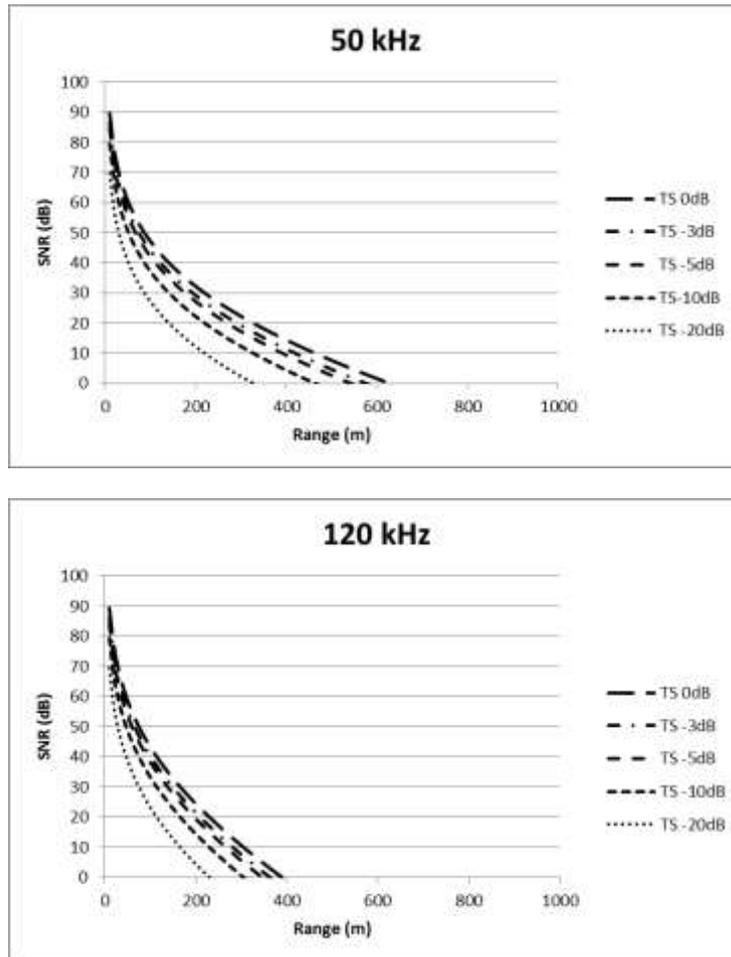
Figure 4. Plots of SNR against operating distance for reflectors with different target strengths for 50 kHz and 120 kHz and NL of 70 dB re 1 $\mu$ Pa.
