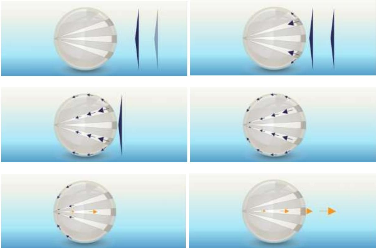
*Figure 2. A sequence of diagrams showing the generation of the second echo by a SonarBell.*
