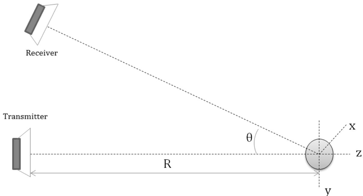
Figure 6. Geometry of the acoustic measurement, with  $\theta = 0^\circ$  for a monostatic setup.
