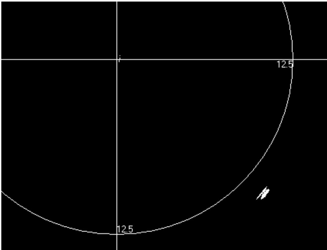
Figure 11. Double echo return from a SonarBell at 13 m distance.
