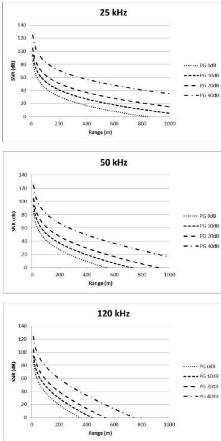
Figure 5. Plots of SNR against operating distance for a reflector with a -5 dB target strength for a sonar with different processing gains (PG) operating at a frequency of 25 kHz, 50 kHz and 120 kHz and NL of 70dB re 1 $\mu$ Pa.
